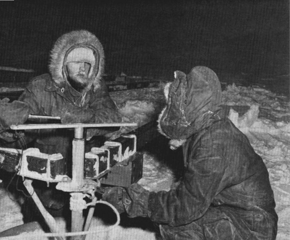
COLD JOB —Navymen stop to make repairs on their crevasse detector while trying to locate safe trail over ice and snow full of deep holes and cracks.
