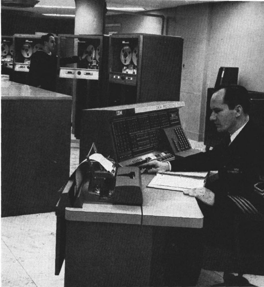
'DRIVER'S SEAT'—A. L. Szymanski, MAC, sits at the 705's console monitoring a data processing run. Sailor in back checks on one of the magnetic tape units.
