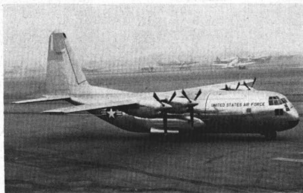
AIR FORCE'S new turbo-prop transport YC-130 can carry 20 tons of cargo and has many new loading features.
