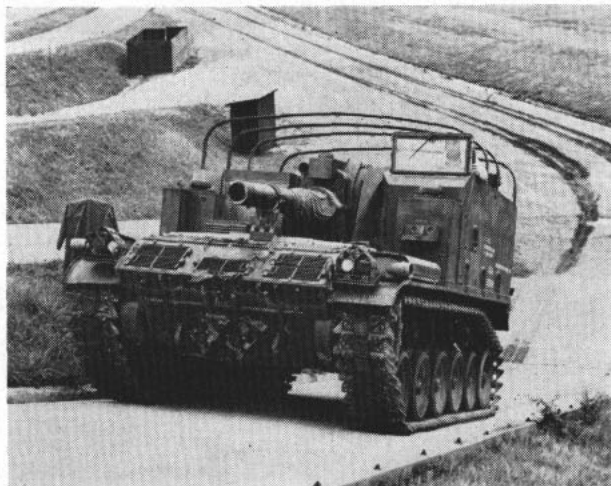
THE ARMY'S 155 MM TANK is the largest of the light tank family, capable of traversing almost any type terrain.
