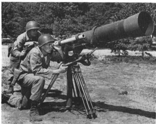
ONE-EYED GIANT —The Army's long-range 100-inch camera has photographed objects as far as 30 miles away.
