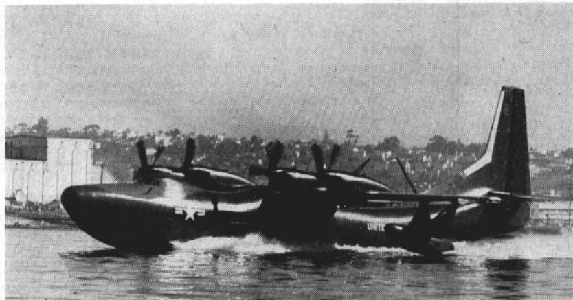
AMERICA'S first turboprop seaplane transport, the Navy's long-range R3Y-1 Tradewind, races down San Diego Bay before taking off on her maiden flight.
