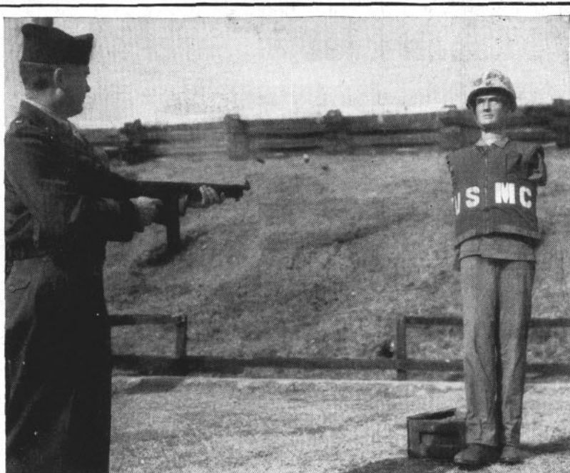
MARINE COLONEL fires .45 caliber submachine gun slugs at point-blank range at a dummy protected by one of the Marine Corps's plastic vests.
