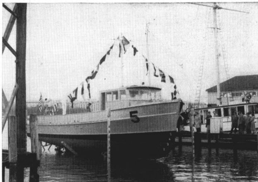
PROTOTYPE of a new minesweeper boat that can be launched from a mother ship and operate in shallow depths, 57-ft. MSB-5 hits the water at Annapolis.
