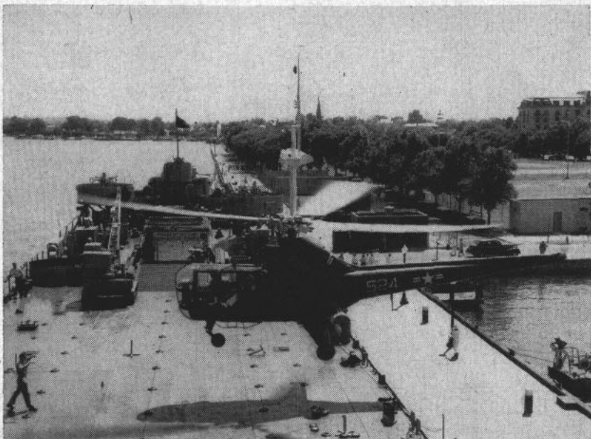
HELICOPTERS can operate easily from the broad deck of the craft. In Korea, one LST has been specially rigged to land 'copters on mine spotting duty.
