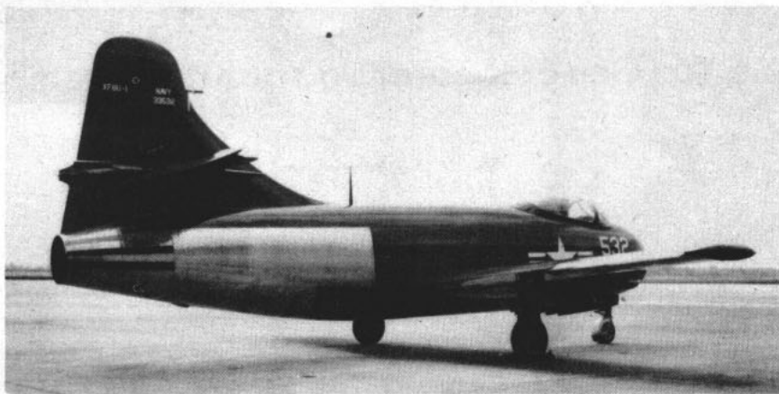
AFTER-BURNER on new version of Navy jet fighter, the XF6U-1 Pirate, boosts its power for short periods. The burner incorporates the principles of ram jet.
