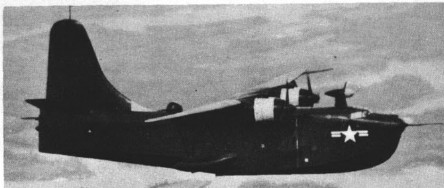
SPREADING its wings on its first test flight the Martin XP5M-1 was designed for the Navy to evaluate new type hull and tail for future long range flying boats.
