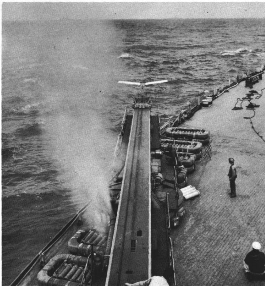
CATAPULTING of radio-controlled target drones from ships at sea is included in training schedule of Reservists who are studying the field of pilotless aircraft.
