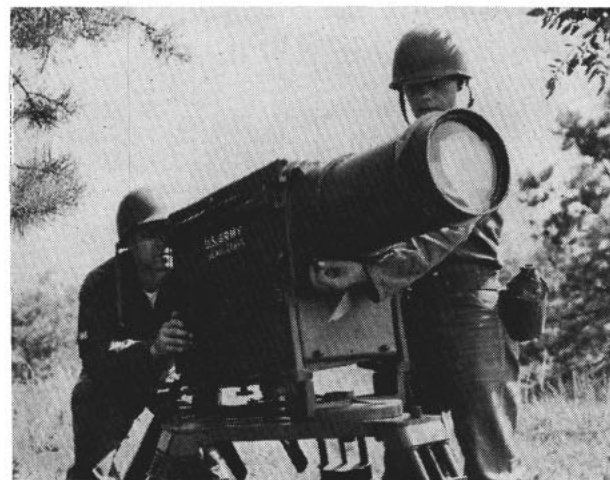
WATCH THE BIRDIE —Signal Corps specialists check telescope, lens barrel of 100-inch reconnaissance camera.
