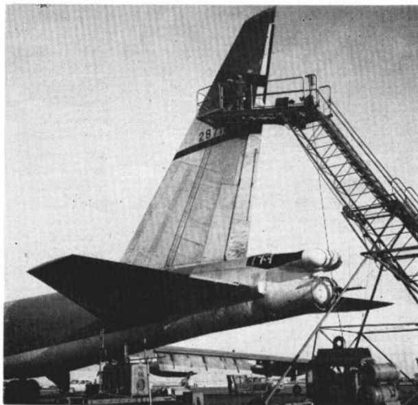
IT'S A LONG REACH for the Air Force ground crew servicing radio gear in tail of B-52 that stands over 48 feet.
