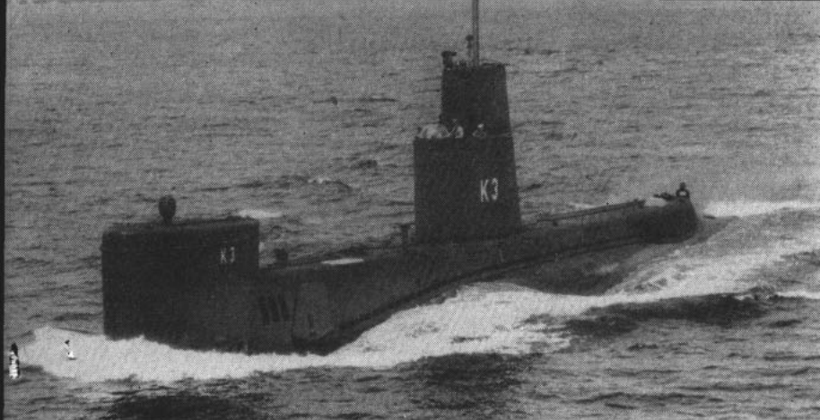
NAVY'S KILLER SUBMARINE of the K-Type makes passage in waters near Pearl Harbor. Boxed-nose contains the latest in electronic listening devices.
