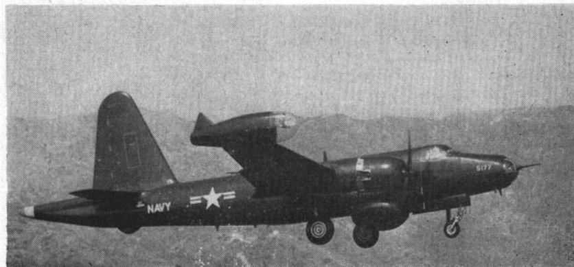
ELONGATED 'stinger tail' on P2V-5 Neptune is latest thing in ASW weapons. It can seek out enemy subs hundreds of feet beneath the ocean's surface.
