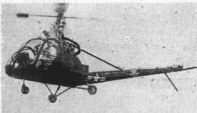
HTE-1 —Specially equipped two-seat training craft. Can carry up to three passengers.
