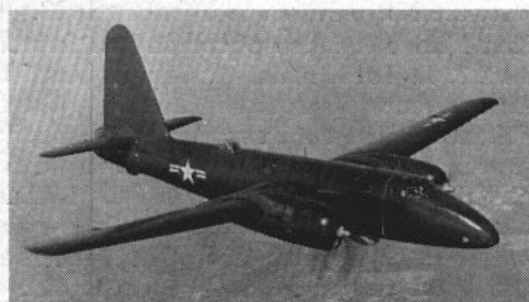
P2V 'Neptune' —Long-range patrol plane, it has take-off weight of 58,000 pounds, maximum speed of 288 mph, range over 3500 miles.
