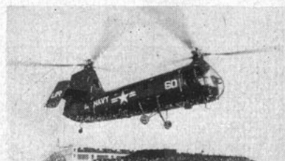
HUP-1 'Retriever' —Designed for shipboard operation. Has outrigger tail fins.
