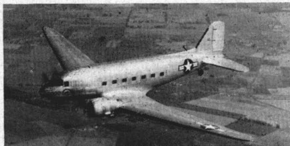
R4D 'Skytrain'—A land-based transport, it can carry up to seven tons. Twin-motored, it has a range of more than 2000 miles.
