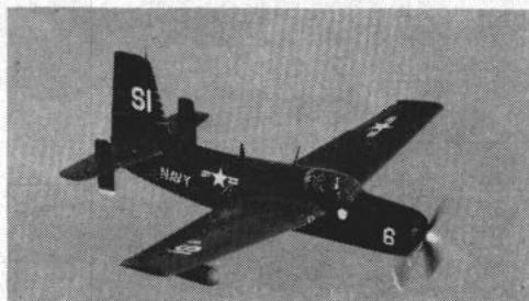
AF-2S 'Guardian' —Anti-submarine plane, it's paired with AF-2W (search) craft. It weighs about 20,000 pounds, has a span of 60 feet. Speed over 300 mph.
