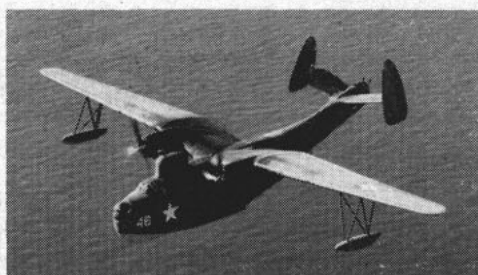
PBM 'Mariner' —Performs general utilities. Not in production now. Span 118 feet, gross weight 56,000 pounds, speed 200 mph. Range over 2000 miles.
