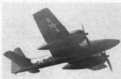
F7F-2 'Tigercat' —Gross weight 13,000 pounds, span over 51 feet. Used in Korea, plane has speed over 425 mph, range of over 1500 miles.
