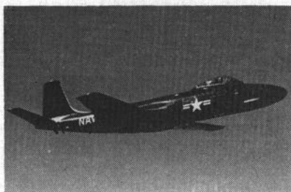
F2H-3 'Banshee' —This is improved version of F2H-2. A single-seat, jet-propelled fighter.
