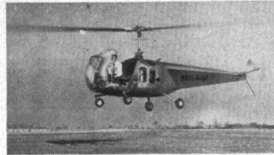
HTL-2 —Designed for training purposes. Features split canopy side-by-side seating.
