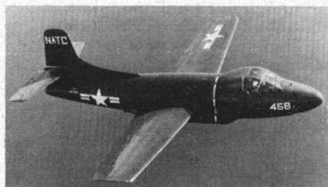
F3D-1 'Skynight' —Jet-propelled, carrier-based, all-weather fighter. It weighs about 27,000 pounds, has a speed in excess of 600 mph.
