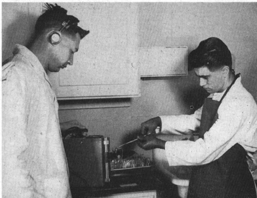
CHECK for radioactivity is made before lab equipment is put away following use. Radiation count must be at a very low level or equipment is washed again.
