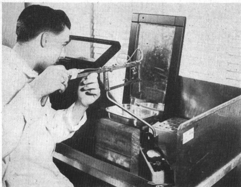
RADIOACTIVE material is measured out by use of a remote control pipette on a radium loading bench. Technician is protected by a heavy lead shield.
