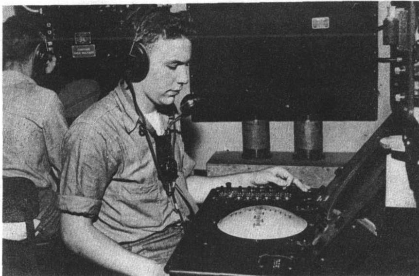
LATEST GCA equipment instantly identifies aircraft and determines altitude of each plane in approach pattern. Device is being tested at NAS, Quonset Point.
