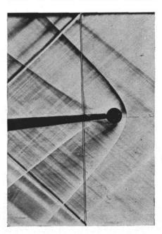
WAVE PATTERN produced by air moving past sphere tested in wind tunnel at supersonic speed is pictured here.
