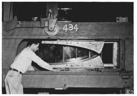
BALLISTIC characteristics of supersonic missiles are tested in wind tunnel at NOL. Optical bench contains mirrors which are used in photographing flow of air.
