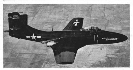
MOST powerful carrier-based fighter plane in world is Navy's new Banshee. Plane can climb 9,000 feet per minute and has top speed of over 600 miles per hour.
