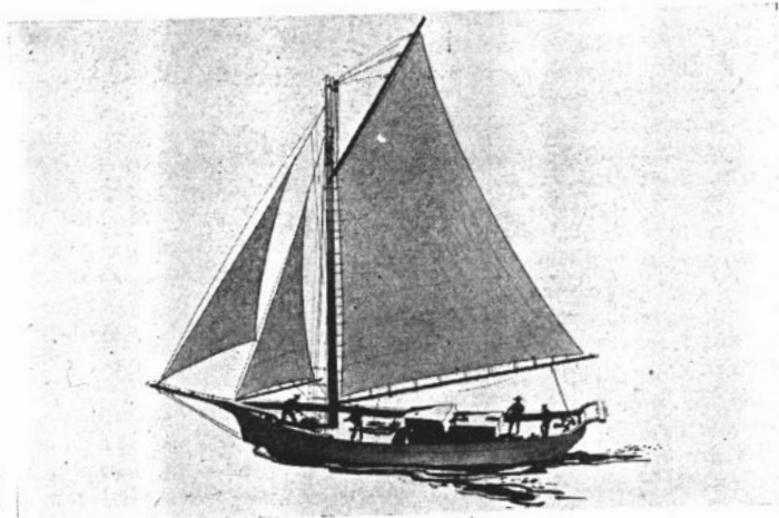
SLOOP: These vessels, most common in the West Indies, are used for all purposes—fishing, freighting, passenger carrying. Its one mast is set fairly near the bow. There is a large mainsail, forestaysail and jib.
