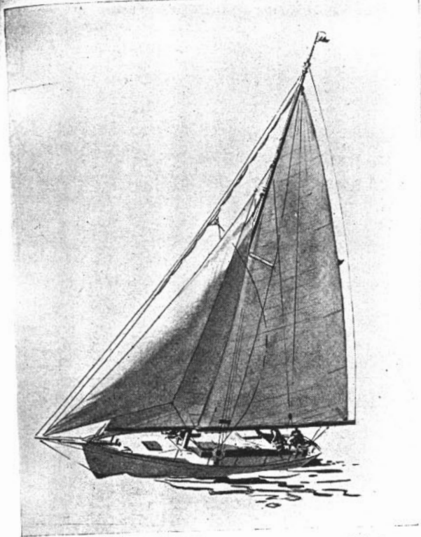
CUTTER-RIGGED YACHT: This is likely to be found in U. S. coastal waters; has forestay-sail and jib set and a third ready to break out.
