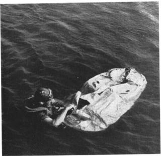
(1) He turns valve on bottle of carbon dioxide and raft inflates in 1 minute. Rafts are standard equipment on Navy single-seat fighters.
