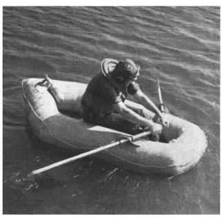
(4) A pair of collapsible oars are stowed aboard the raft. The pilot inserts oars in oar-locks and he is away.
