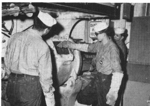
MOLTEN METAL is poured into bull ladle. Right: Molder prepares to check for pouring temperature.
