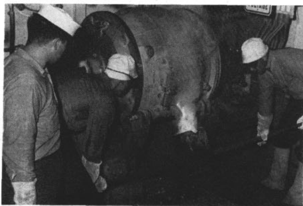
MOLTEN METAL is poured into bull ladle. Right: Molder prepares to check for pouring temperature.
