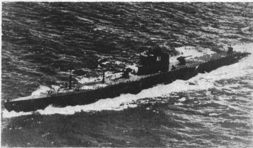
LARGEST U.S. SUBMARINE— USS Argonaut (APS 1) had an over-all length of 381 feet, a beam of 33.8 feet and displaced 4080 tons when submerged.
