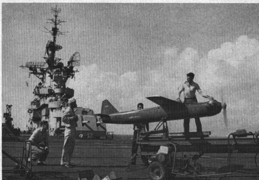
CREWMEN make final adjustments on radio-controlled drone on flight deck of USS Tarawa (CVA 40) before drone is launched as target for ship's guns.
