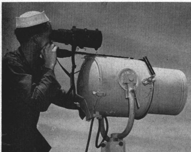
SEARCHLIGHT has special hood, filter, viewer for sending 'invisible' light messages. Man (right) holds small viewer.
