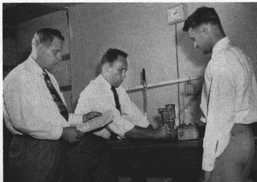
O. H. WELPER, EN1, I. B. Pierson, EM1, and F. T. Duba, IC1, are creating and observing nature of tracks made by alpha particles—nuclei of helium atoms.
