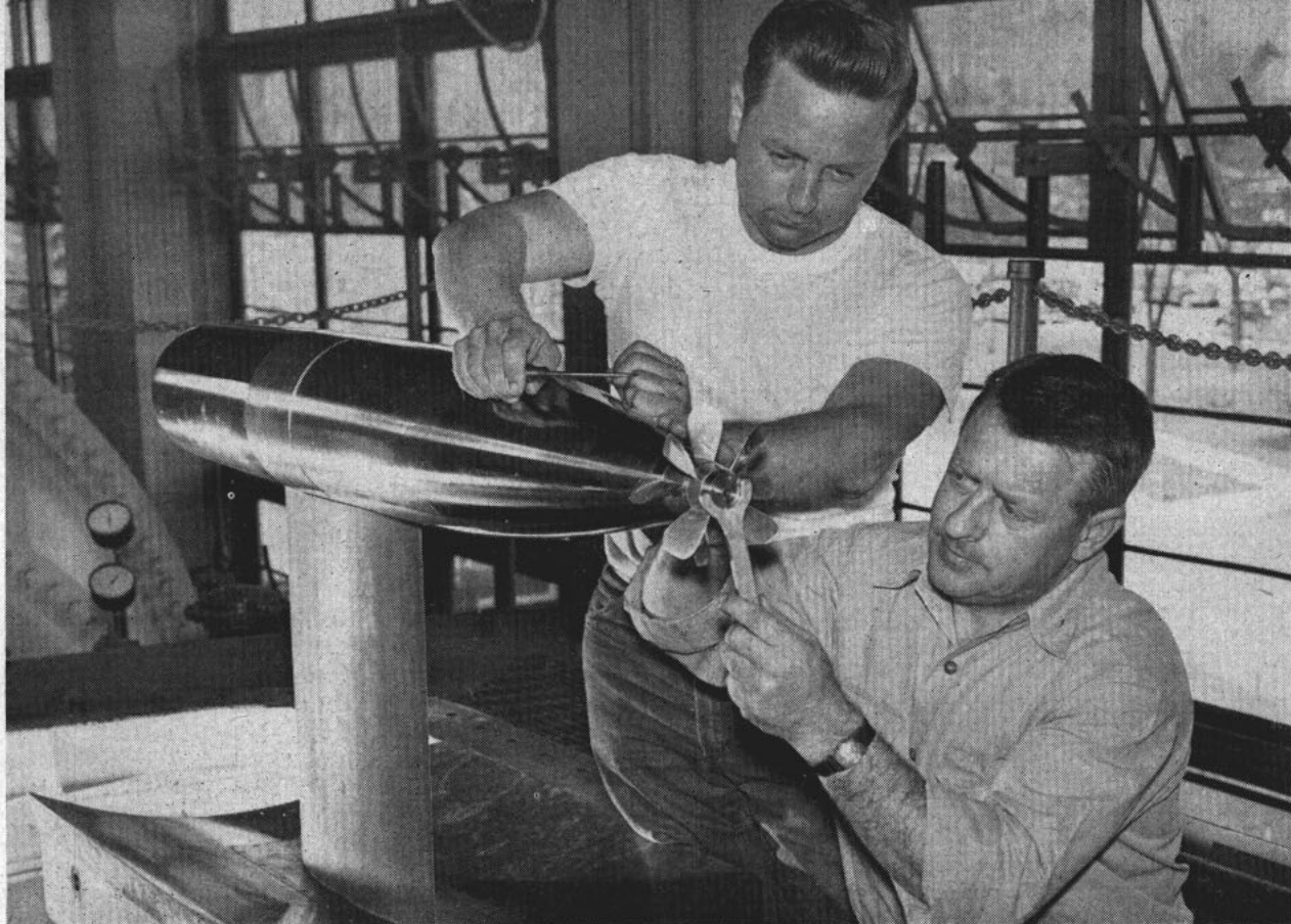
TECHNICIANS fit prop to desired shape. It is then mounted in water tunnel for turbulence tests at varying speeds.
